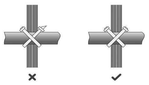
If cables are to be bent, bind them first but do not tie cable ties within the bend to avoid stress on the cables, which
