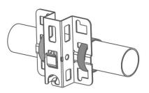
b. Align the host with bracket and mounting plate to the bracket on the pole, and tighten the M8×20 screws to complete installation.
