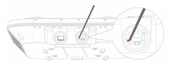
Before pressing the reset button, please remove the waterproof joint first. Refer to the Chapter 3.5 Connecting Cables for more information.
