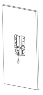
b. Align the host with bracket and mounting plate to the bracket on the wall, and tighten the M8x20 screws to complete installation.
