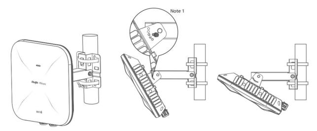
b. When the angle of the access point is properly adjusted, secure the access point with M4x10 screws in the position shown in Note 1.
