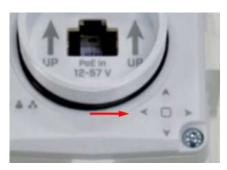
The arrows will light up and show the direction where to turn the unit. The goal is to reach the 0.4 - 0.8 degree range, where the signal is at its peak.
