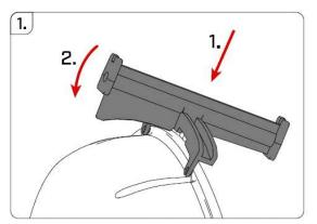
Attach the AIM tool under angle as it is shown in picture [1], then continue to rotate until it locks in place with a click sound [2].
