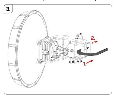
4. Attach the assembly to the pole.
