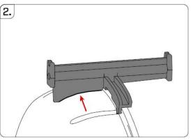
Make sure that the lower fin of the tool fits tightly against the cover.
