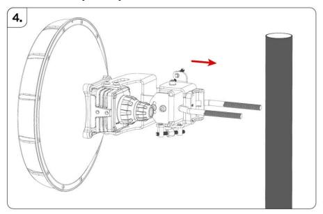
5. Add mount bracket and use two  $13\ \text{mm}$  nuts to secure the device.
