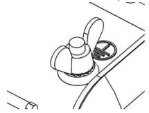
The device includes a grounding connection (marked  $\equiv$ ).
