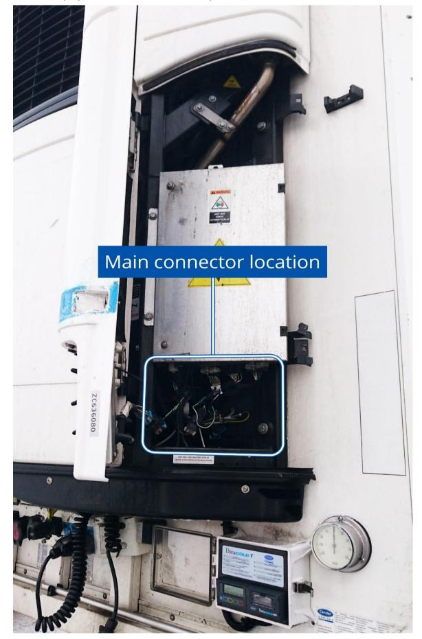
Figure 4 The main connector location
